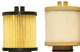
When installed both filters seal radially, however the sealing point is different for each. The OE style filter seats and seals in the ID of the flange in the filter housing. This design requires an extended area at the bottom of the filter which fits into the flange area. The radial seal is formed as the filter is seated.
