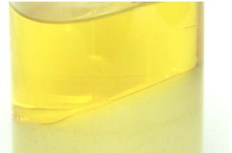
This means the media itself is chemically resistant to the flow of water. As the fuel water mixture attempts to pass through the media, the water content is stripped out. The water molecules are more dense than those of the fuel and collect in the bottom of the housing to be drained out based on the manufacturer's suggested guidelines. Because the WIX filter does not use the membrane construction, bleed holes are also not required to vent the air than can become trapped under such coverings.
