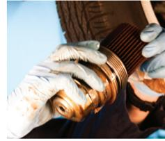
**8** Clean both the filter housing cap and housing. Examine for damage such as a cracks, breaks, or damaged threading. Check the O-ring seatings, making sure they are undamaged and clean. Replace damaged components if needed. While removing the used O-ring, note its proper placement on the cap or housing.
