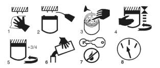
It is important to install all filters in accordance with the manufacturer's recommended procedures to avoid any unnecessary problems. Always observe the markings for proper tightening, lubricating, and other instructions on the outside of the filter can.
