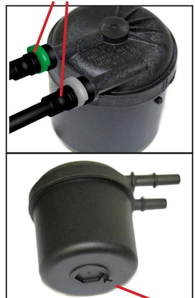
Loosen filter cradle bolt and twist filter slightly to unseat from cradle.
