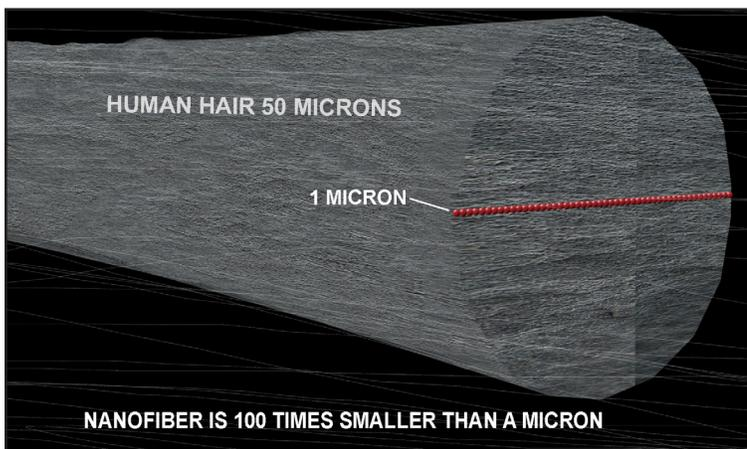
The added nanofibers dramatically improve filter efficiency and capacity making the filter suitable for fine filtration needs. This new fuel water separator is available and ready to meet the demands of new engine technology by providing superior protection and filtration performance.
