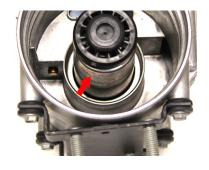
Because the 33899 fuel water separator seals at the post, the extra extension is not required.
