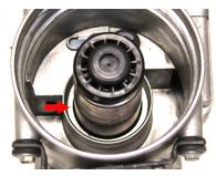
The WIX 33899 filter creates a radial seal around the center post of the housing.
