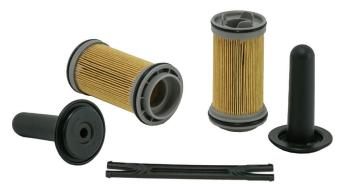
Covering a wide range of popular truck and other commercial applications, the WIX W74B191 filter is suitable for on-road and off-road use. Supplied as a kit which includes a filter element, a filter element removal tool, and an equalizing element, this offering replaces the supply module's Urea filter in many SCR dosing systems.
