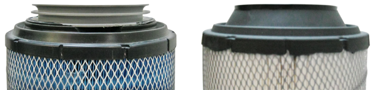
A view of the water skimmer in the filter tops (ours on right). Dirty-wet air flows through the air inlet in the housing, up the angle on the filter, and over the corner. This helps channel water out of the air that drops to the bottom of the filter to the drain hole.
