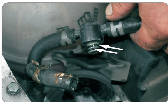
Install new sealing rings onto regulation valve element
