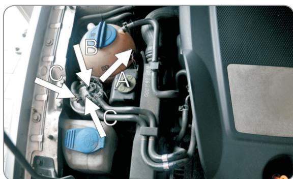
Remove the fastening clamp (A) and regulating valve (B), loosen the fuel hose bands, remove hoses (C)
