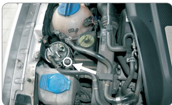
Loosen the filter clamping ring screws, remove used filter
