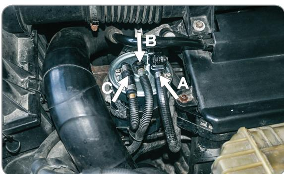
**EN** Fix fuel heater cycle regulator (A), fuel outlet connection (B) and connect the feeder cable (C)
