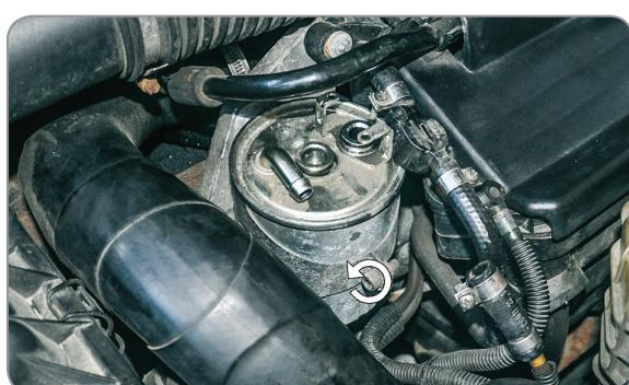
EN Loosen damping ring fastening the filter, take filter out
