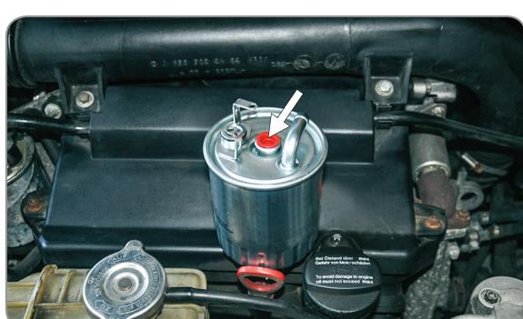
EN Remove safety plug from filter (A) fill filter with clean diesel oil, place filter in clamping ring
