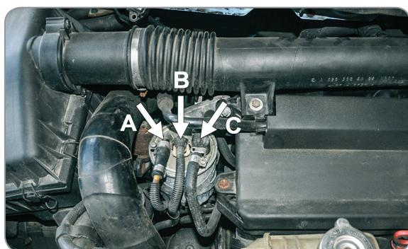
EN Disconnect the feeder cable (A and B), disconnect the fuel heater cycle regulator (C)
