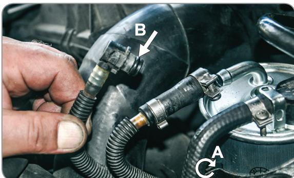
**EN** Tighten clamping ring fastening the filter (A), fix a new gasket on the fuel outlet connection (B)
