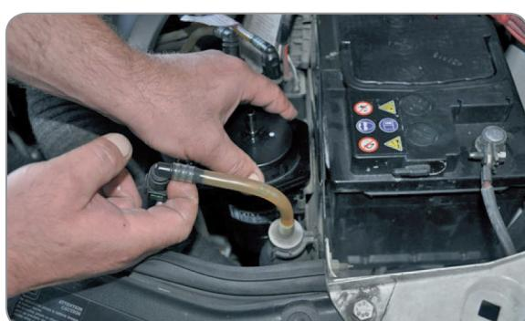
EN Gently remove fuel filter off the bracket, fix new filter on it
