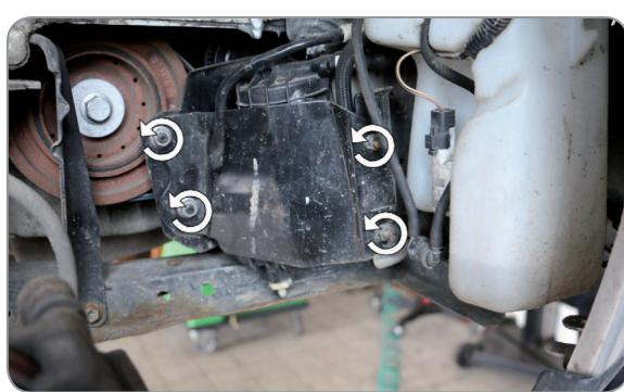
(EN) Loosen the screws of the filter housing
