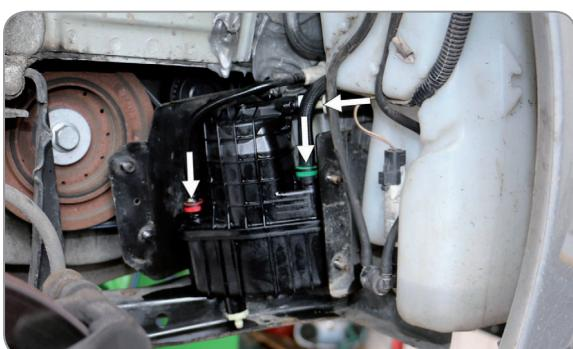
**EN** Install filter in seat, remove safety plugs, connect fuel pipes
