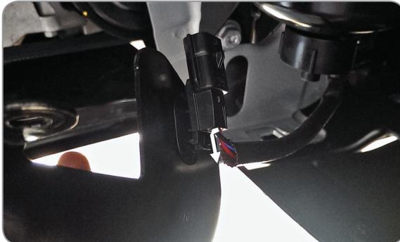
**(EN)** Disconnect the electric circuit
