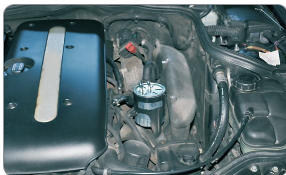
EN Loosen filter clamping ring and remove filter from the clamping ring
