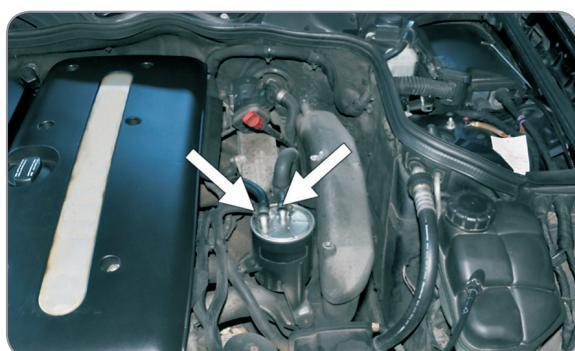
EN Use screw driver to loosen band clips and remove fuel hoses
